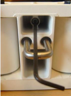
Locate the hex adjustment screw behind the XY Assembly. Use a 3 mm hex tool to adjust the XY Lock release for optimal lock and minimal slack in transport mode.
