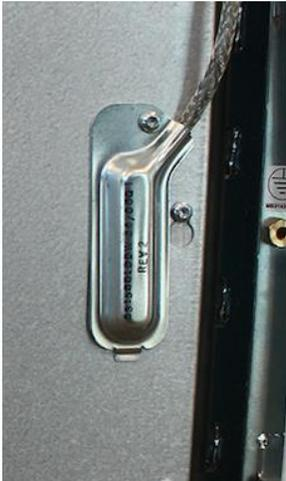
Unscrew the fixing screw for the cover for the PCIe (GFI) cable and remove the cover for the PCIe cable. Shown on the left. Unplug the PCIe cable and unscrew the FEP Cover's ten fixing screws.
