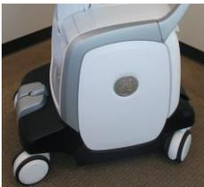
The side covers are fastened with two “click” locks, located at the lower end of the cover. To remove the side covers:
