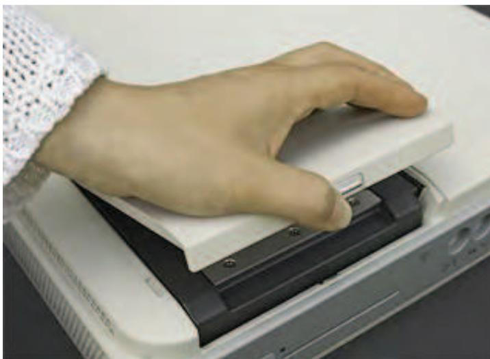
Installing the battery
