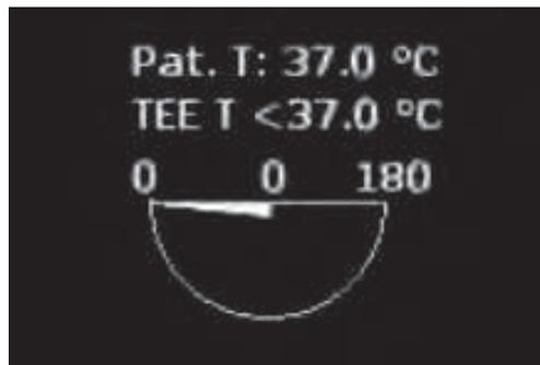
A less-than sign (<) after **TEE T** indicates that the transducer's distal tip temperature is below the patient temperature (**Pat. T**) assumed by the system, which is either 37°C (98.6°F) or the temperature you entered.
