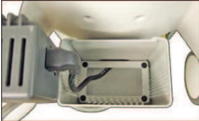
2. Slide the adapter into the tray, top side out.
