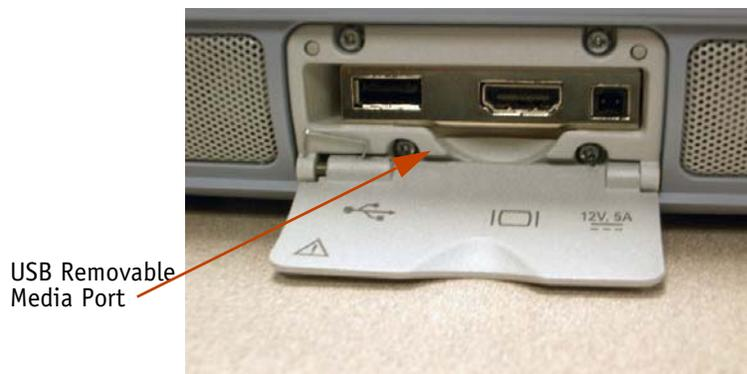
Figure 4-3. Scan Engine Example: Rear View - Removable Media Port
