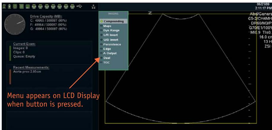
**Figure 3-6. Menu on LCD Display**
