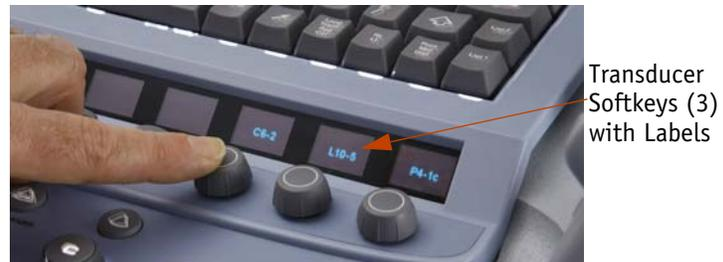
**Figure 6-5. MTP Transducer Softkeys**
