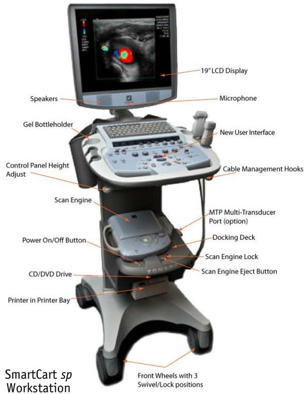
Figure 2-3. z.one *ultra sp* Convertible Ultrasound System
