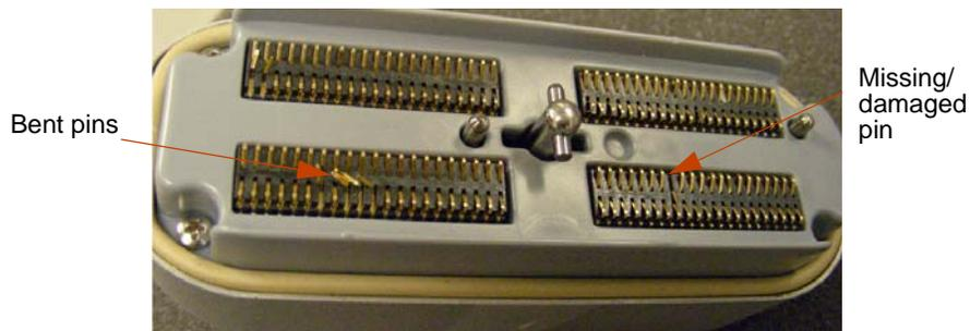
**Figure 14-30. Bent, Broken, or Missing Pins on Transducer**
