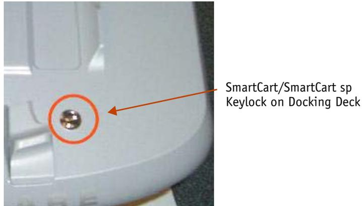
Figure 2-9. SmartCart/SmartCart *sp* Keylock Location
