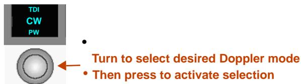
**Figure 7-22. Doppler Mode Softkey (far right on softkey panel)**
