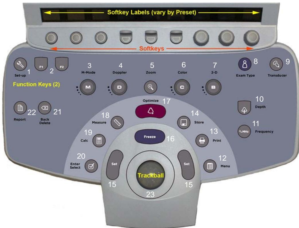
Figure 3-2. SmartCart *sp* Control Panel
