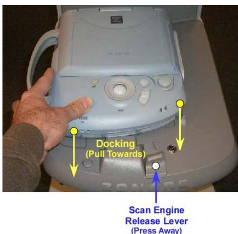
Figure 2-8. Docking/Undocking Scan Engine/Scan Module
