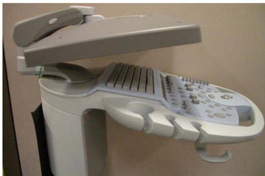
Figure 2-15. SmartCart/SmartCart sp LCD Display Position for Transport
