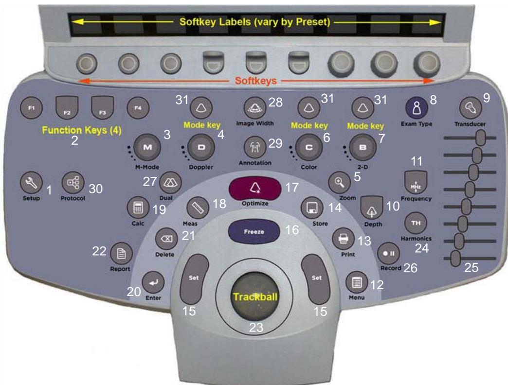
Figure 3-1. SmartCart Control Panel
