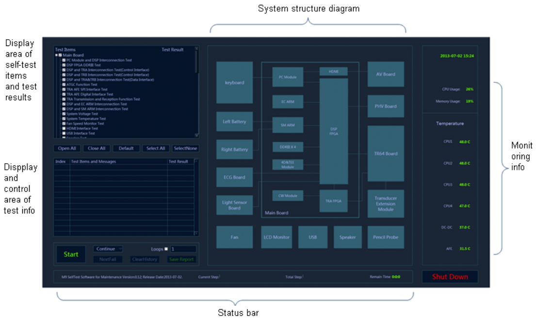
Figure 10-2 Maintenance self-test interface
