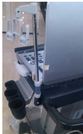
Figure 9-5 -Installing probe hook assembly Install storage tray. See Chapter 0 for details. Install the option modules if there are relevant modules for options: probe extend module, audio/video extend module. See Chapter 9.2.2 and Chapter 9.2.3 for details.
