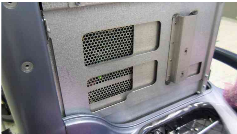
Figure 7-1 check green LED inside CPS
