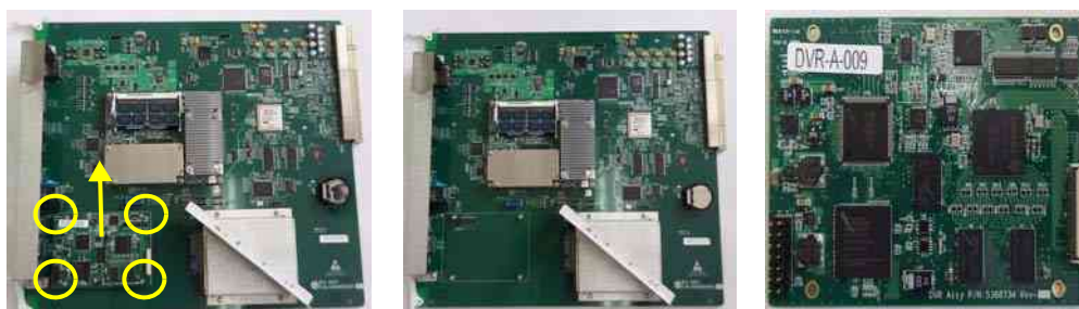
Figure 8-78 Drawing up the DVR
