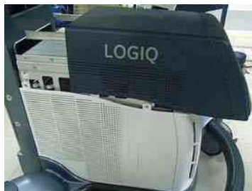
Figure 8-137 Pulling out top cover
